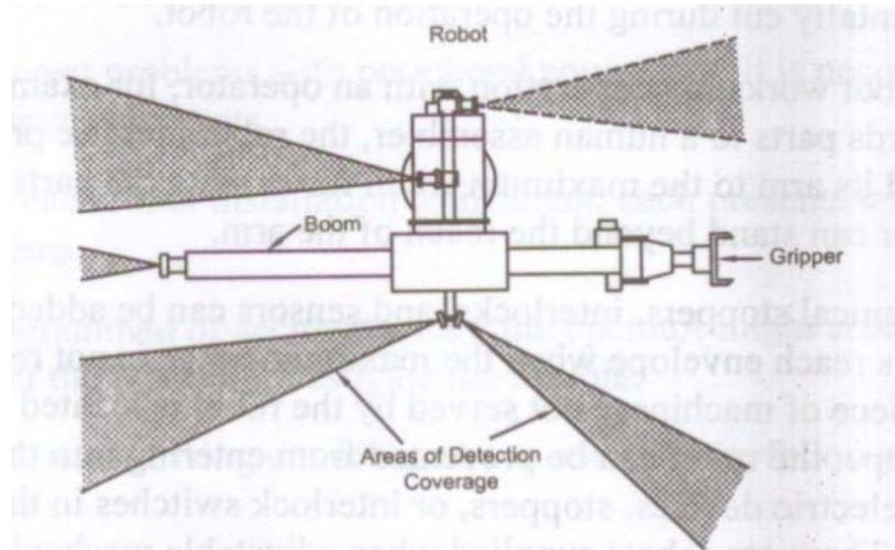
Figure 3.3 : Robot Transducers with Coverage Areas
