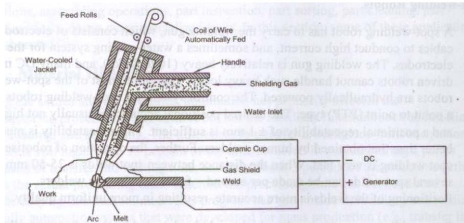
**Figure 3.1 : Insert Gas Shielded Arc Welding with a Continuous Wire Fed as Electrode**
