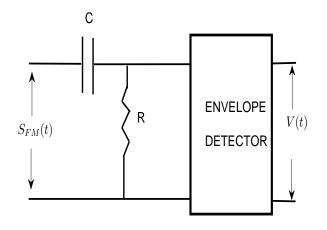
Fig. 2. Using an envelope detector for FM demodulation
