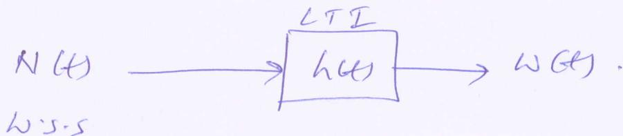
Let  $N(t)$  be a wide sense stationary (W.S.S) random process which is the input to a LTI filter characterized by its impulse response  $h(t)$ .
