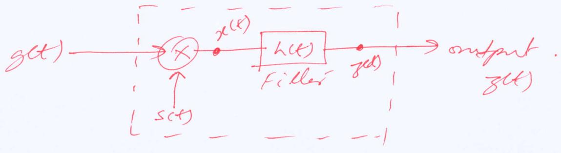
where  $s(t) = \cos(\omega_f t - \eta k t^2)$ , and  $h(t) = \cos(\omega_f t + \eta k t^2)$ .
