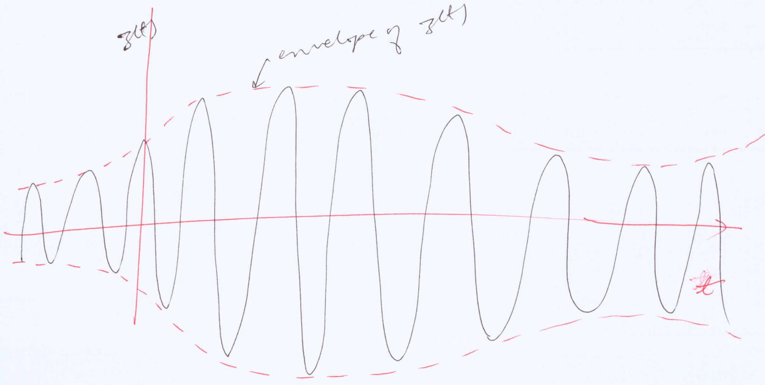
$$\begin{aligned} \therefore \text{envelope of } z(t) &= |\tilde{z}(t)| \\ &= \left| \frac{e^{j\omega_0 t}}{2} \int_{-\infty}^{\infty} g(z) e^{-j\omega_0 z} dz \right| \\ &= \frac{1}{2} \left| \int_{-\infty}^{\infty} g(z) e^{-j\omega_0 z} dz \right| \\ &= \frac{1}{2} |G(f = \omega_0 t)| \end{aligned}$$
