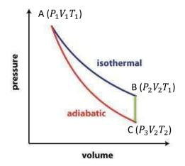
$$\delta q_{rev,AB} = \frac{nRT_1}{V} dV \quad \Rightarrow q_{rev,AB} = nRT_1 \ln \frac{V_2}{V_1}$$
