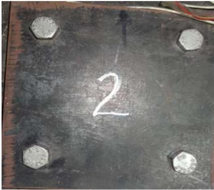
Figure 6 (a) Retrofitting plate with four bolts of 10mm diameter,
