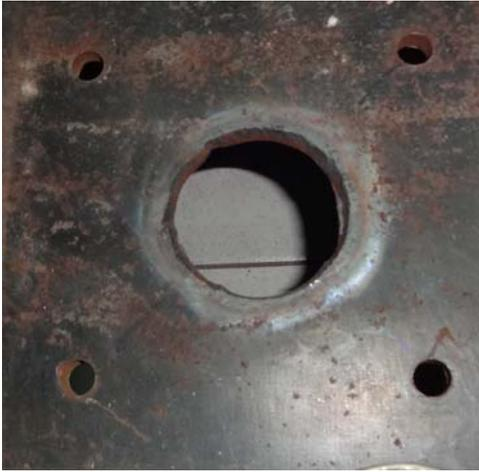
Figure 5 Damage location created at the 15<sup>th</sup> panel of the plate
