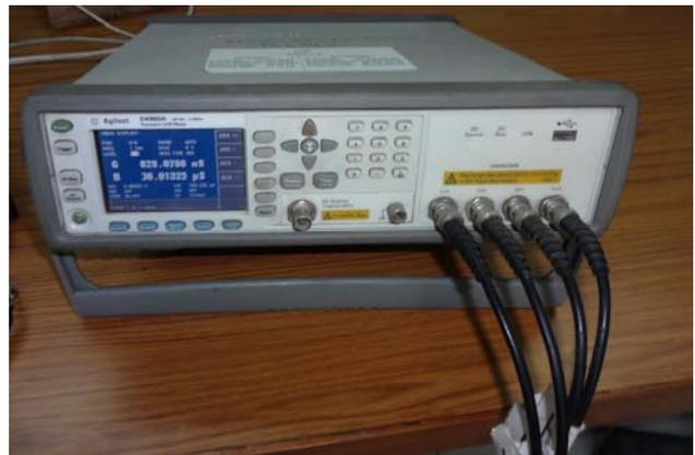
Figure1 Electrical impedance analyzer (LCR meter Agilent E4980)
