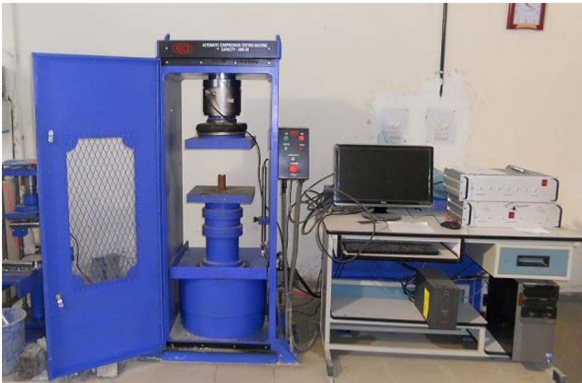
Figure2.7 Compression Machine used for testing.
