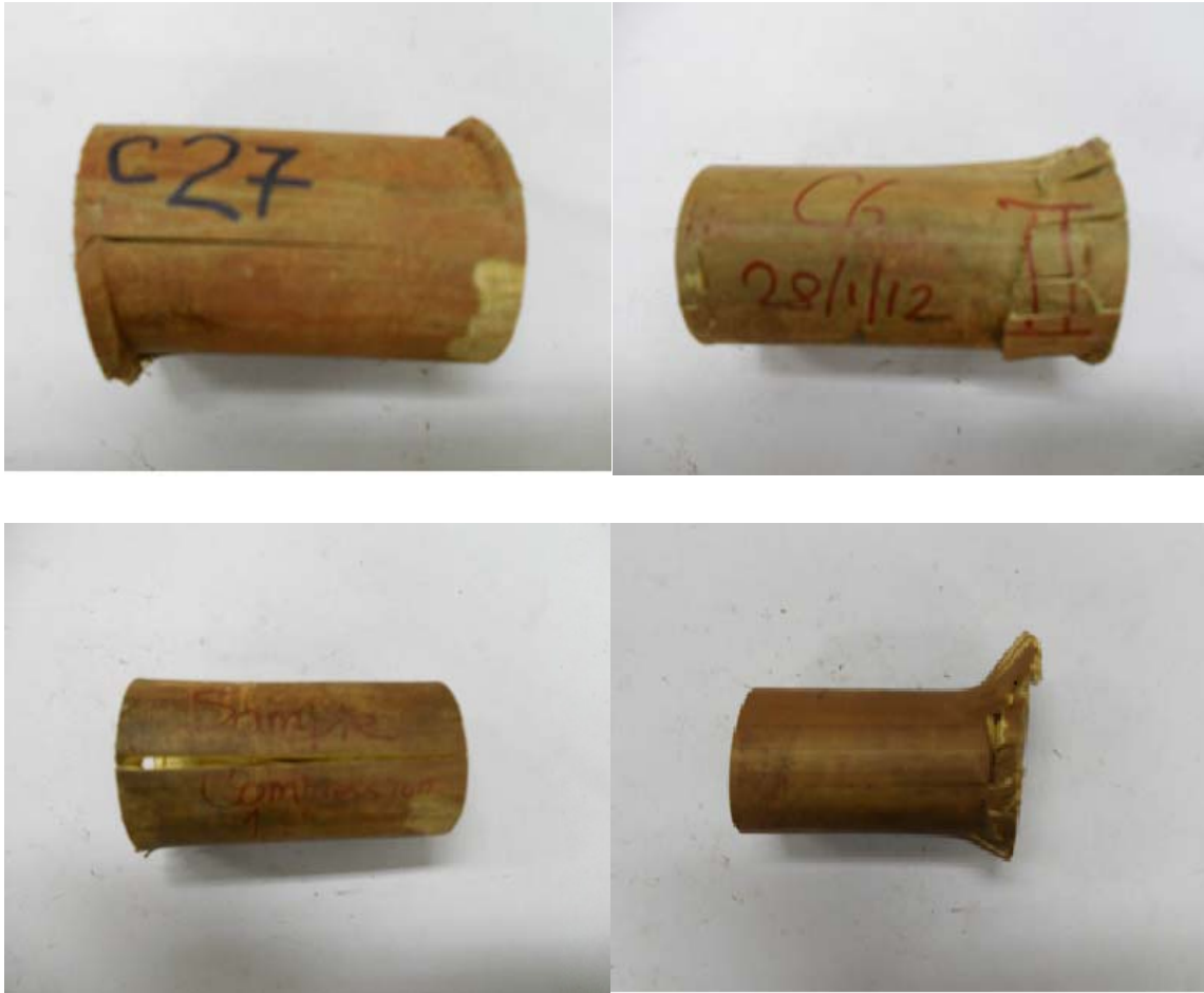
Figure 2.8 Some Photographs showing modes of failure of the compression specimens. The specimen at the bottom left failed in pure cracking whereas the one at the top right failed in crushing predominantly, very similar to the one at the bottom right. The specimen at the top left seems to fail in both cracking and crushing.
