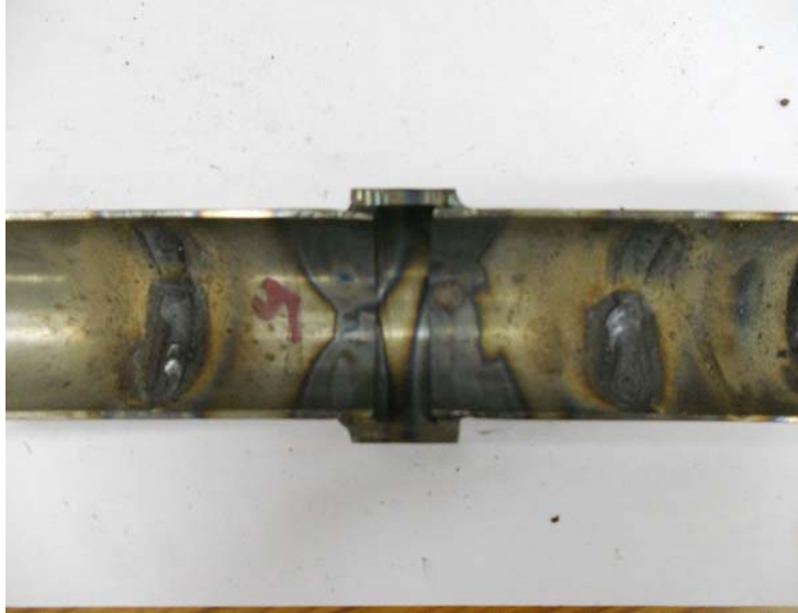
Figure5.2 Close up photograph showing serrations in the collars made with the intention of increasing the friction capacity
