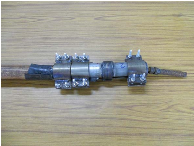
Figure5.3 Photograph showing the failure of joint test. Upon looking carefully it can be observed that the rubber started to tear out and slip
