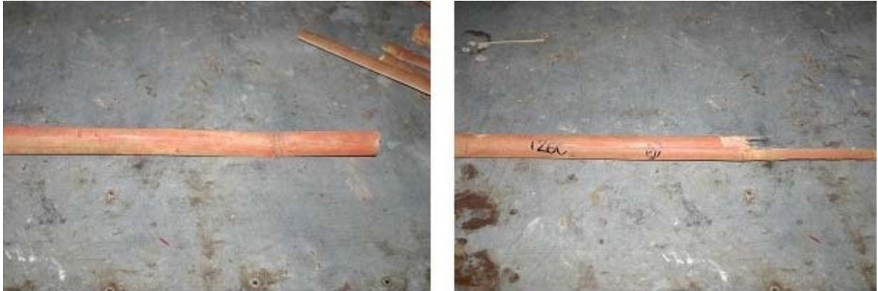
Figure 3.2 Tensile Test Specimen before testing (Left) and after testing (Right). The specimen has been ripped off from its joint.
