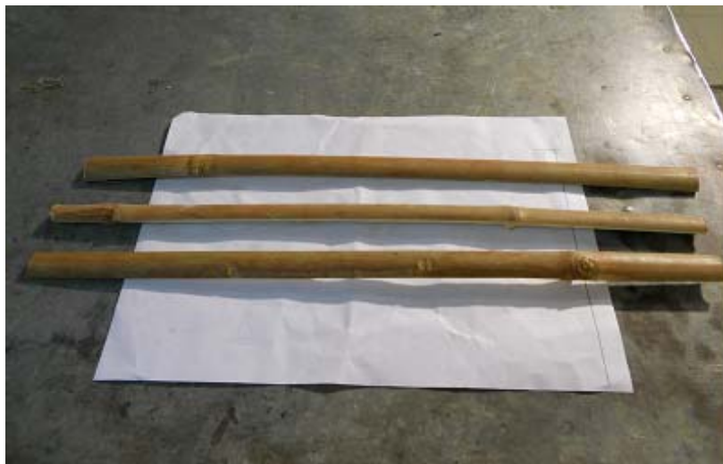
Figure3.1 Specimens used for tensile testing. The specimens were cut from a whole bamboo piece circumferentially into four equal parts
