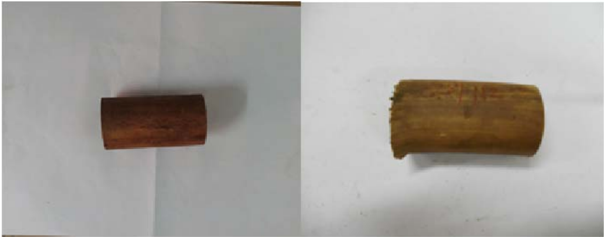
Figure2.6 Specimen before Compression test (Left) and after Compression test (Right). The specimen on the right shows the crushing of the left most end.
