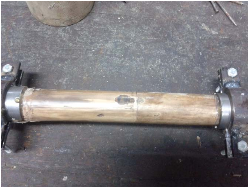
Figure 6.8 Failure of Araldite Bamboo sample
