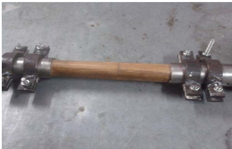
Figure 6.4 Failure of Simple Bamboo sample
