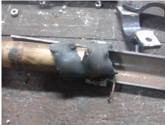
Figure 6.5 Failure of Tube-Tyre Rubber Bamboo sample
