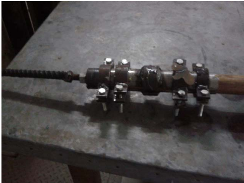
Figure 6.6 Friction Joint of Araldite Bamboo sample
