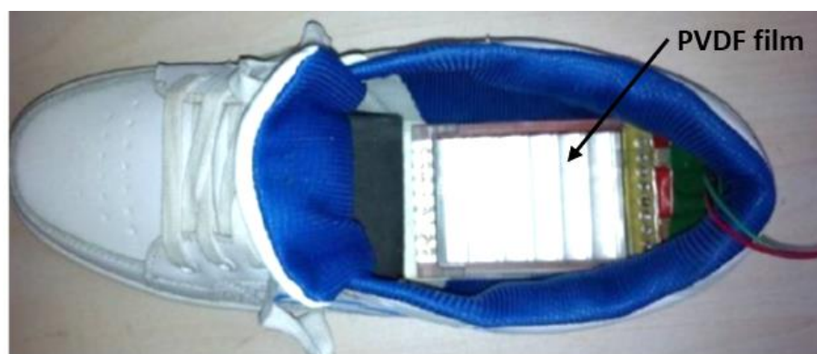
Figure 2.9: PVDF film installed in the human shoe (Zhao et al., 2014)
