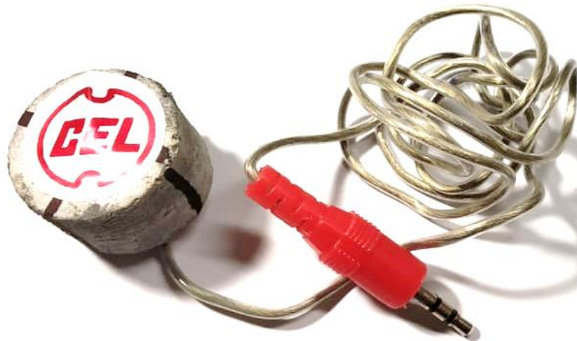
Figure 2.5: Concrete vibration sensor (CVS) (SSDL, IIT Delhi)
