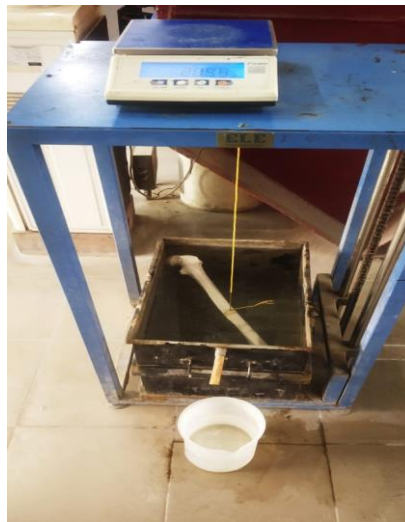
Figure 3.6: Laboratory setup for measuring specific gravity of bone
