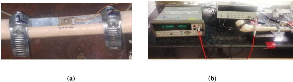
Figure 3.2: (a) NBPS clamped on bone using two jubilee clamps
