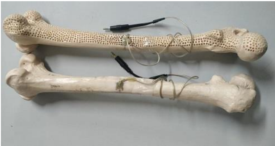
Figure 3.10: DBPS configuration of PZT on healthy and osteoporotic bones.
