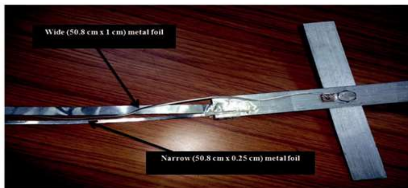
Figure 2.6 Specimen with wide and narrow foils attached
