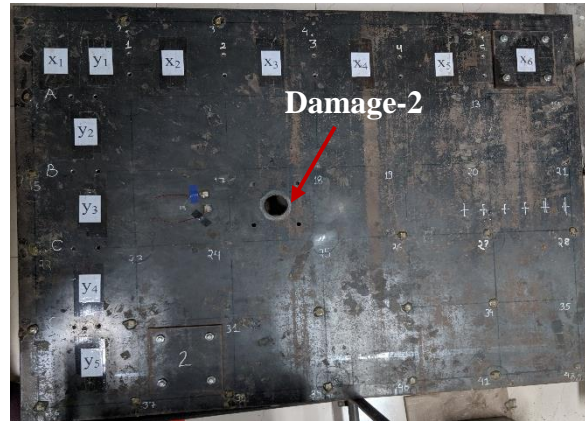
Figure 4.10: Damage-2 on the steel plate
