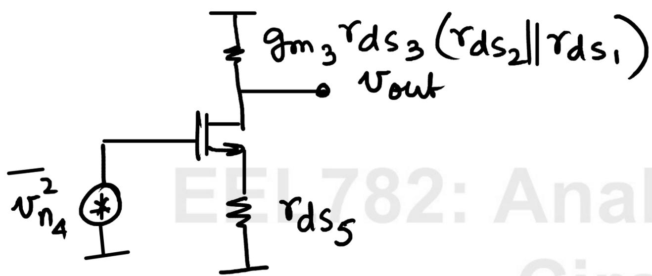
$$\overline{v_{out}^2} = \frac{\overline{v_{n4}^2}}{r_{ds5}^2} \left[ g_{m3} r_{ds3} (r_{ds2} \parallel r_{ds1}) \right]^2$$
