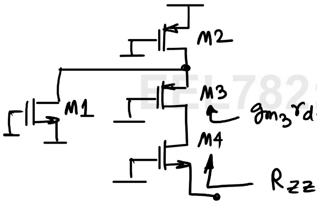
$$R_{zz} = \frac{r_{ds4} + g_{m3} r_{ds3} (r_{ds2} || r_{ds1})}{1 + g_{m4} r_{ds4}}$$
