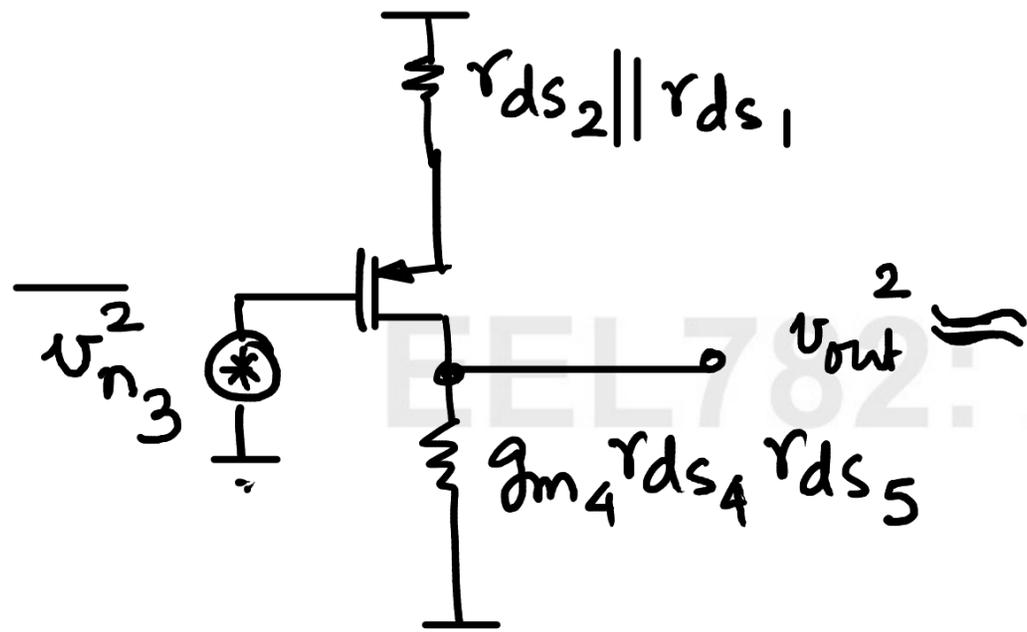
$$v_{out}^2 \approx \frac{v_{n3}^2 (g_{m4} r_{ds4} r_{ds5})^2}{(r_{ds2} || r_{ds1})^2}$$
