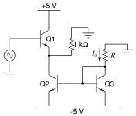
**Design:** 1. Design a current mirror circuit with  $I_0 = 1$  mA,  $r_o = 100$  kΩ. Assume that the early voltage of the given transistor is 100 V, and  $\beta$  is 200. Choose an appropriate value for the resistor.
