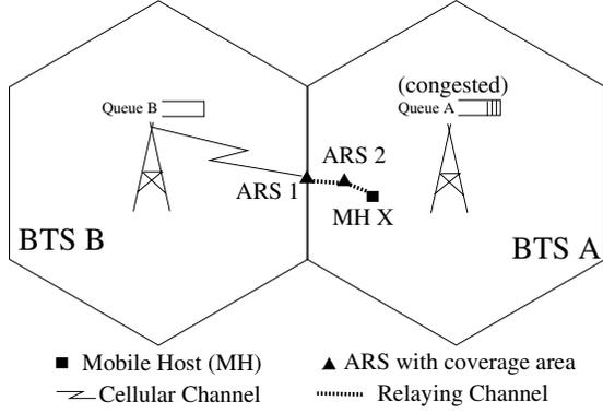
Fig. 1. A relaying example. The relaying route is established from MH X in a congested cell A to a BTS in the non-congested B through two ARSs.
