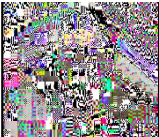
(b) Video frame during a bad channel state
