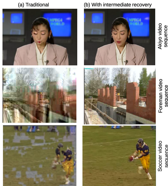
Figure 14: MDC-MPT performance example: Two sample frames of Akiyo, Foreman, and Soccer sequences
