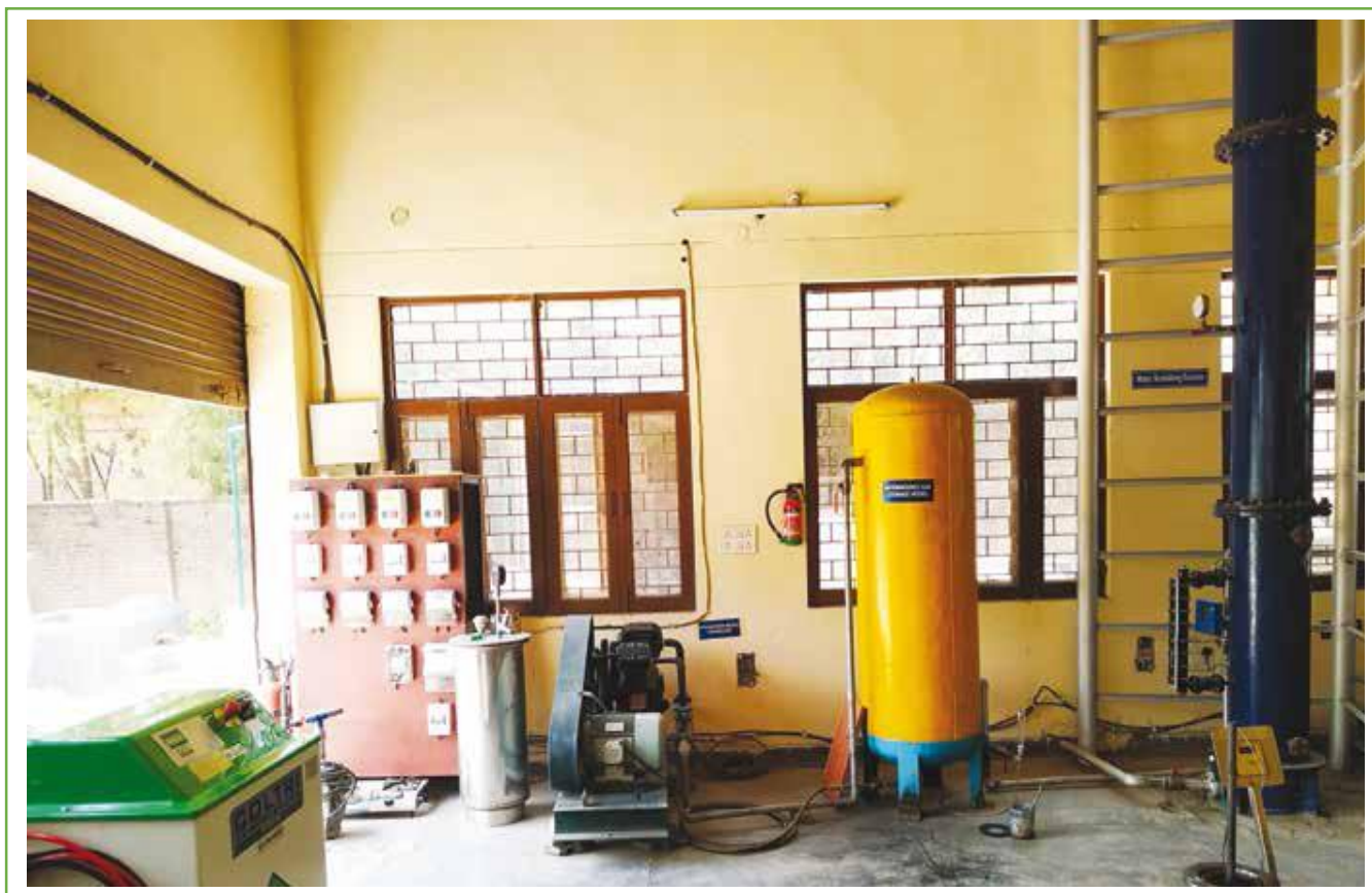
Fig. 7 A 25 m 3 /h capacity CBG plant at Biogas production and Enrichment Lab, CRDT, IIT Delhi.
