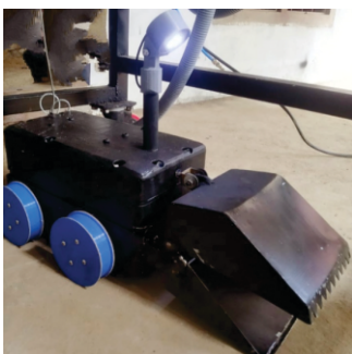
PIPE BOT FOR CLEANING
